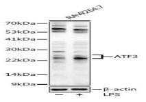
Western blot analysis of extracts of RAW264.7 cells, using ATF3 antibody at 1:1000 dilution.Raw264.7 cells were treated by LPS at 37°C for 8 hours.<br/>br/>Secondary antibody: HRP Goat Anti-Rabbit IgG at 1:10000 dilution.<br/>br/>Lysates/proteins: 25ug per lane.<br/>br/>Blocking buffer: 3% nonfat dry milk in TBST.<br/>br/>Detection: ECL Basic Kit .<br/>br/>Exposure time: 90s.
