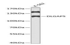
Western blot analysis of extracts of K562 cells, using DLGAP5 antibody at 1:1000 dilution.<br/>Secondary antibody: HRP Goat Anti-Rabbit IgG at 1:10000 dilution.<br/>Lysates/proteins: 25ug per lane.<br/>Blocking buffer: 3% nonfat dry milk in TBST.<br/>Detection: ECL Basic Kit .<br/>Exposure time: 90s.
