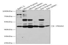
Western blot analysis of extracts of various cell lines, using PIGM antibody at 1:1000 dilution.<br/>Secondary antibody: HRP Goat Anti-Rabbit IgG at 1:10000 dilution.<br/>Lysates/proteins: 25ug per lane.<br/>br/>Blocking buffer: 3% nonfat dry milk in TBST.<br/>Detection: ECL Basic Kit .<br/>br/>Exposure time: 120s.
