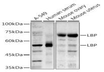
Western blot analysis of extracts of various cell lines, using LBP antibody at 1:1000 dilution.<br/>Secondary antibody: HRP Goat Anti-Rabbit IgG at 1:10000 dilution.<br/>Lysates/proteins: 25ug per lane.<br/>br/>Blocking buffer: 3% nonfat dry milk in TBST.<br/>br/>Detection: ECL Enhanced Kit .<br/>Exposure time: 90s.
