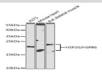
Western blot analysis of extracts of various cell lines, using HSP20/HSP20/HSPB6 antibody at 1:1000 dilution.<br/>
