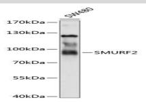
Western blot analysis of extracts of SW480 cells, using SMURF2 antibody at 1:1000 dilution.<br/>
