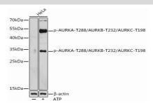
Western blot analysis of extracts of HeLa cells, using Phospho-AURKA-T288/AURKB-T232/AURKC-T198 antibody at 1:1000 dilution. Hela cells were treated by ATP at 30 °C for 1 hour. <br/>
