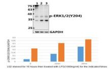
Western blot (WB) analysis of p-ERK1/2 (Y204) pAb at 1:500 dilution Lane1:L02 starved for 16 hours whole cell lysate(40ug)
