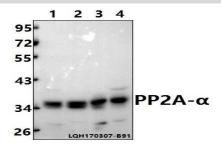
Western blot (WB) analysis of PP2A- $\alpha$  (T301) polyclonal antibody at 1:500 dilution
